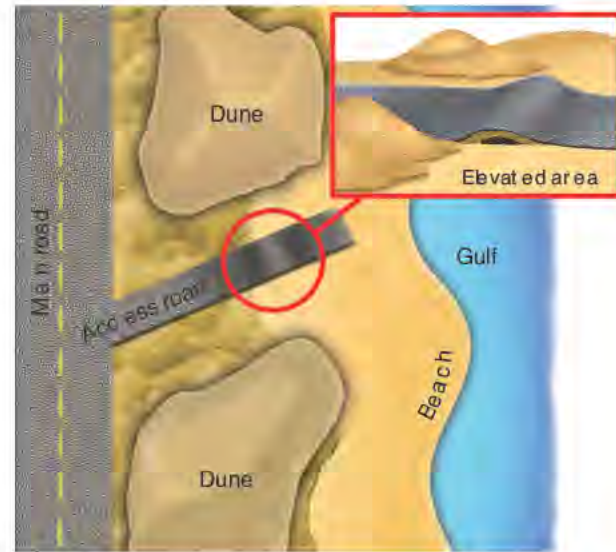
Figure 27. Elevating beach access roads at beach juncture.
